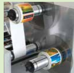
Rewinding to finished rolls
